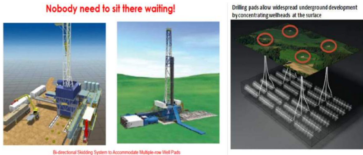
Figure 1.21 Efficient subsurface penetration and minimal surface impact as a result of the multi well pad system (courtesy of CNPC).
